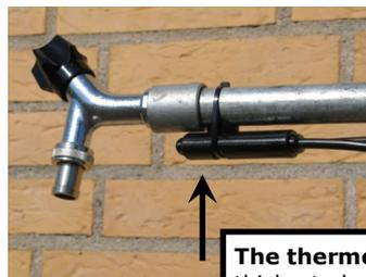
**The thermostat** is placed in the thickest plastic-part. Place the thermostat on the coldest end of the pipe. The heating cable and the thermostat must be covered by the insulation. If the product is used on a plastic pipe, always use aluminium tape over the heating cable and thermostat onto the pipe. This will move more heat from the cable to the pipe and ensure the frost protection.
