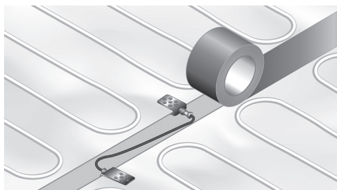
Fig. 9. Installation of earth connections
