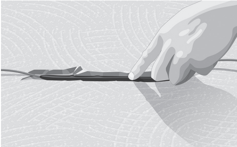
Fig. 2. Groove for joint of cold and heating cable
